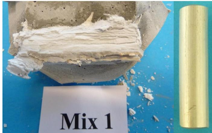
Figure 20: Example of aluminium reinforcements corroding in conventional concrete Reproduced from [13]
